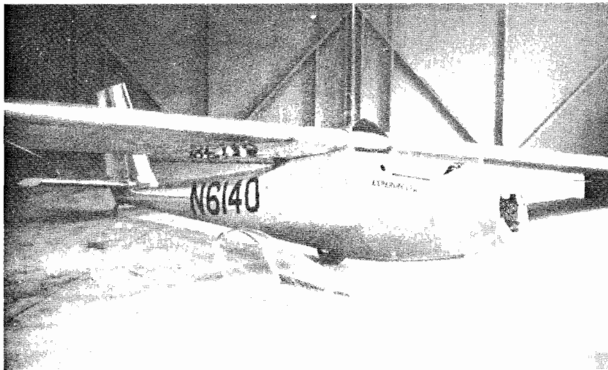
Another Air Cadet construction project is the Pacific D-8 glider, shown with canopy and nose cone removed.
